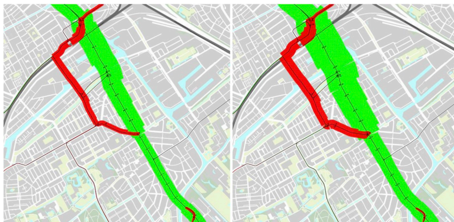
Fig. 2. Comparison between predicted ridership effects of a frequency increase without crowding (left) and with crowding (right) effects incorporated (derived from Van Oort et al., 2016).
