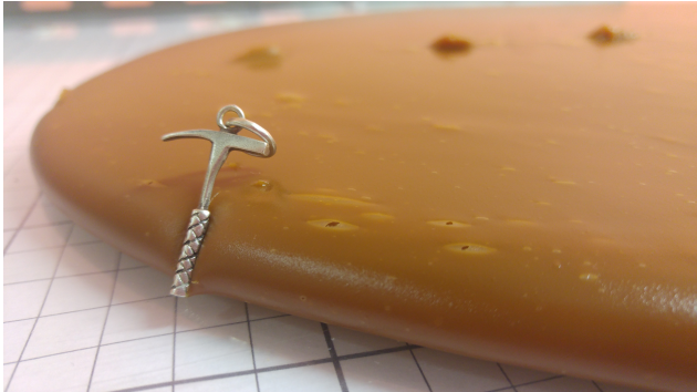
Figure 4.1: Close up of the flow front of manjar. It shows smooth edges and elongated bubbles due to strain. Small hammer of 3 (cm) length for scale, and the square grid on the surface represents an area of 1 (cm 2 ) per square.
