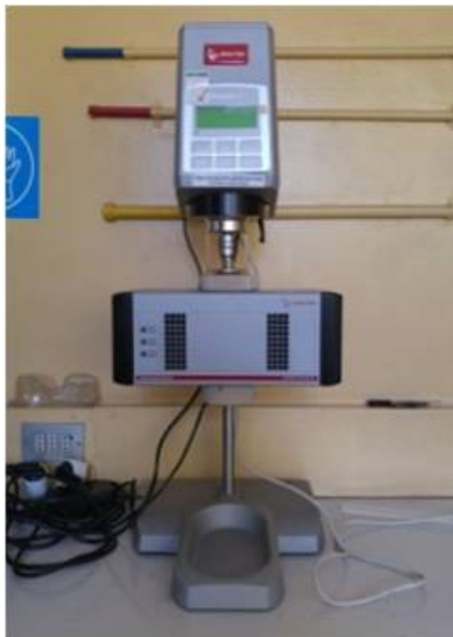
Figure 3.6: Rotational rheometer Anton Paar used in this work. Photo by the autor.
