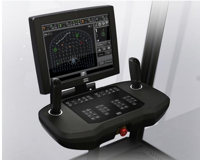
Figura 2-12 Rig Control System (RCS 5). Epiroc.
