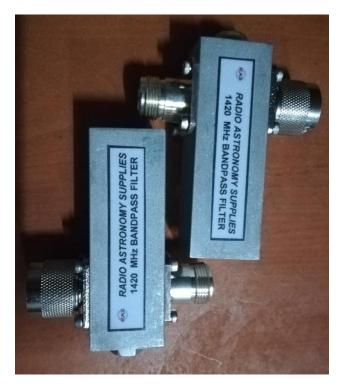
Figure 5.22: Radio Astronomy Supplies bandpass filters.
