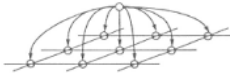
Figure 2.7: Precedence conditions. The point on the top represents the block that will be extracted and the points in the bottom represents the nine blocks that have to be extracted before the extraction of the upper block.
