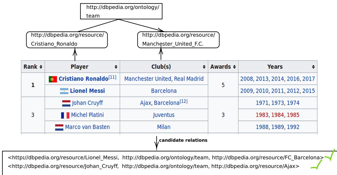
Figure 1.8: Extracting relations from tables according to Muñoz et al. [29]
