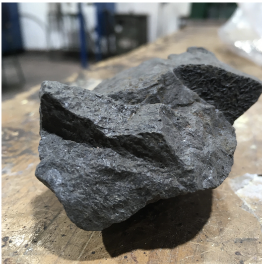
(a) Fractured copper slag sample
