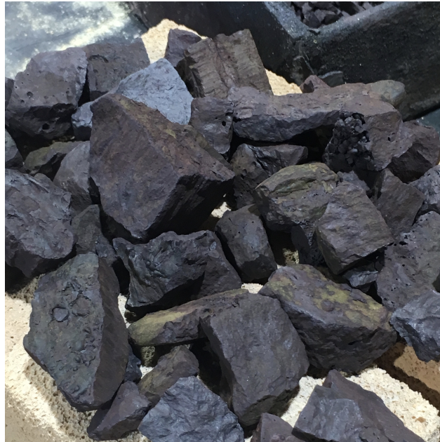
Figure 6.2: Oxidized slag samples with flat sides
