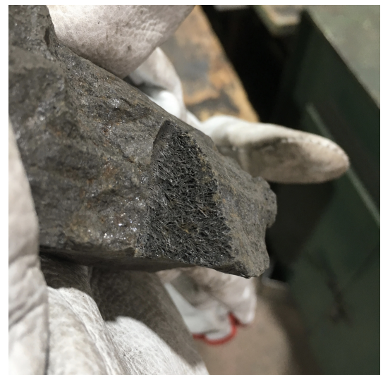
(b) Copper slag sample with stringy fracture
