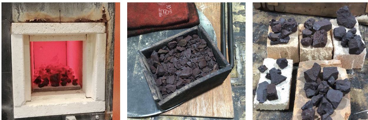
(a) Copper slag at 800°C inside the furnace (b) Small copper slags cooled after cooked (c) Large copper slags cooled after cooked
