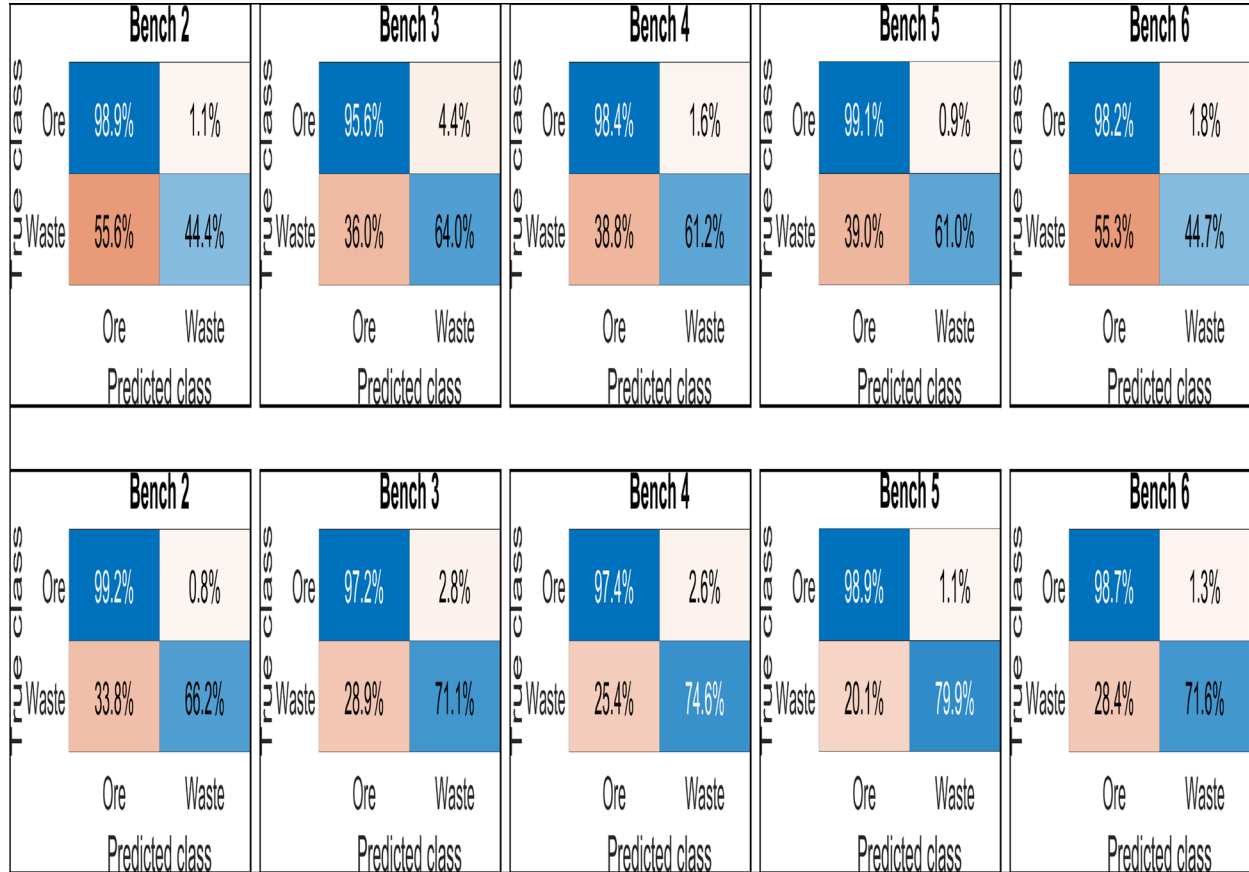
Figure 9. Confusion Matrix for Case Study 1. From left to right: Benches 2–6. Top: Structured sampling. Down: Adaptive sampling using Cut-off grade 1.012%.
