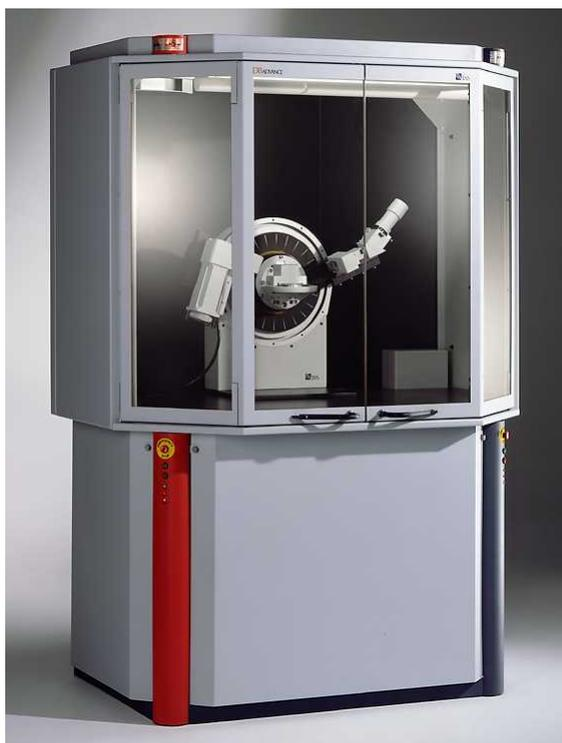
Figura 5.13: Difractor de rayos X, Bruker, D8 Advance.
