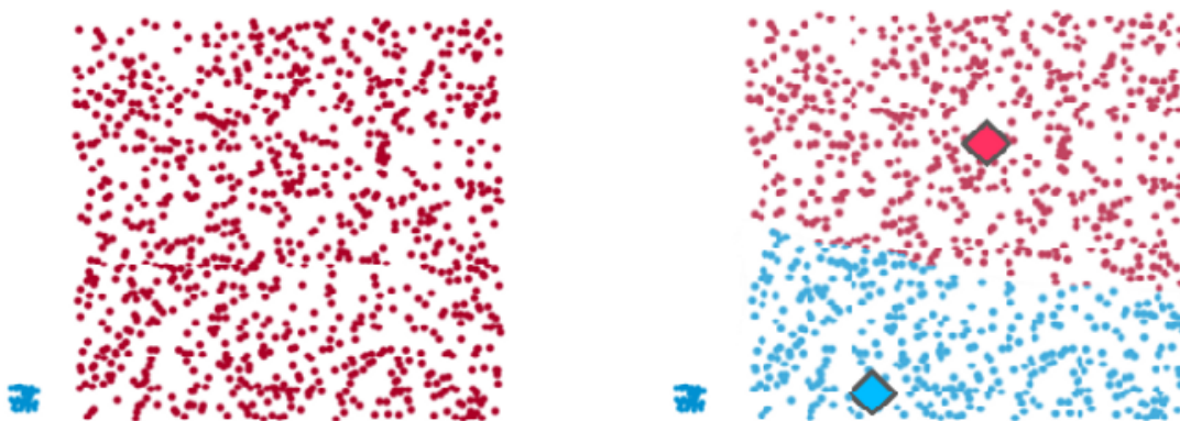
Figure 4.6: Example where the third assumption is not fulfilled. At the left, the raw data is presented and, at the right, the results after using K-Means with 2 clusters are shown. K-means fails to separate the small group with the rest of points. Ref. [51]
