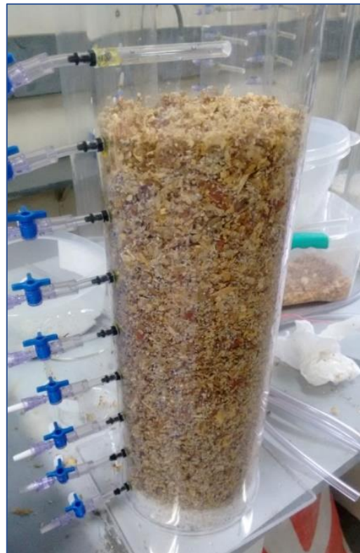
Figure 9: DAS column before starting the experiment (mixture of wood shavings and clam shells). On the left side, 9 sampling ports can be observed (blue three way valves). The distance between sampling ports was 5 cm.
