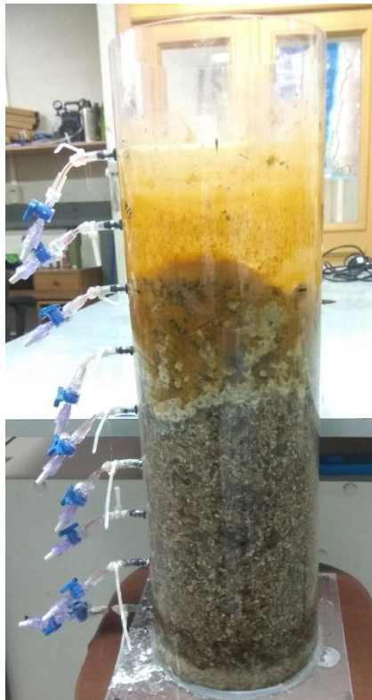
Figure 15: Mussel shell-DAS column at experiment B.2 right before the solid sampling campaigns. The iron (orange) and aluminum (white) precipitation fronts can be observed. Notice that some schwertmannite (orange precipitates) reached deeper in the column using some preferential paths created on the walls but the two precipitation fronts were better defined in the column core (away from the walls).
