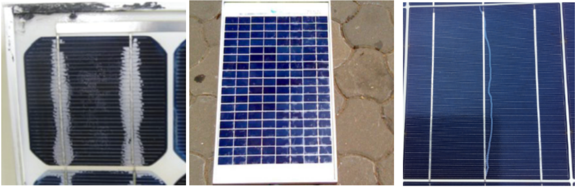
Figure 2.12: Delamination of EVA encapsulant detected by visual inspection.
