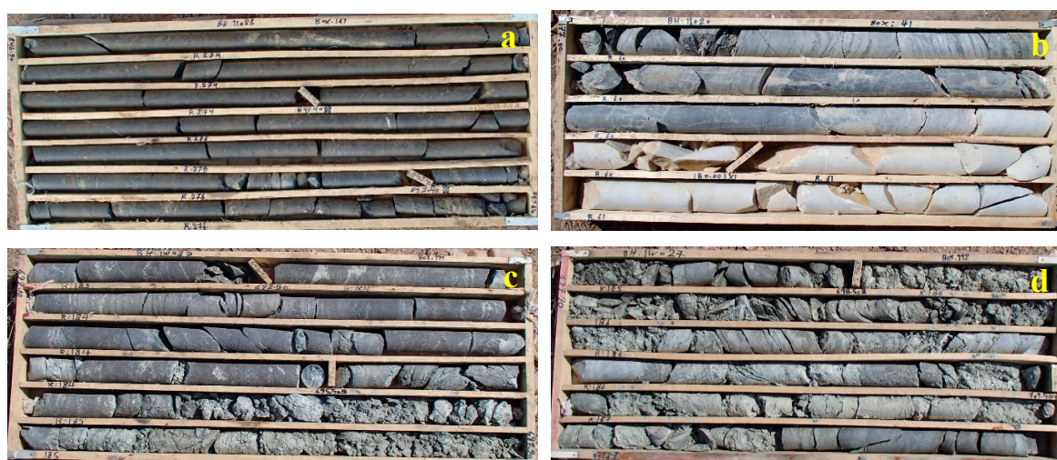
Figure 6. Different types of lithology in the Gol-Gohar iron ore mine (GGIOM). (a) High-grade magnetite, (b) amphibolite, (c) gneiss, and (d) magnetite in schist.
