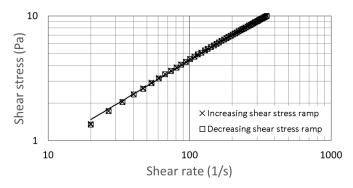
**Figure 2.** Rheogram corresponding to the water-sodium carboxymethyl cellulose (CMC) solution used in Experiment 13. The solid line is the best fitting curve to the measurements, given by  $\tau = 0.194\dot{\gamma}^{0.678}$ , with a correlation coefficient  $R^2 = 0.99834$ .
