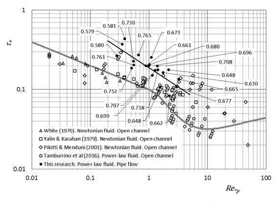
**Figure 5.** Condition of incipient motion presented in the standard Shields diagram with data corresponding to laminar flows of Newtonian and power-law fluids. The grey line is the Rouse–Mantz fitting to the movement threshold condition. The experimental points corresponding to the incipient condition in a pipe flow (this research, black filled circles) show the value of the flow index. The black line is the threshold condition obtained from Equation (14).
