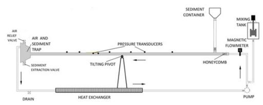
Figure 1. Sketch of the experimental setup.
