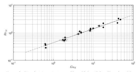
**Figure 4.** Condition of incipient motion in terms of the modified particle Reynolds number and the modified Galileo number. Continuous line corresponds to the best fit of the data. Segmented line is the relationship  $Re_{*p} = 0.434 \sqrt{Ga_K}$ .
