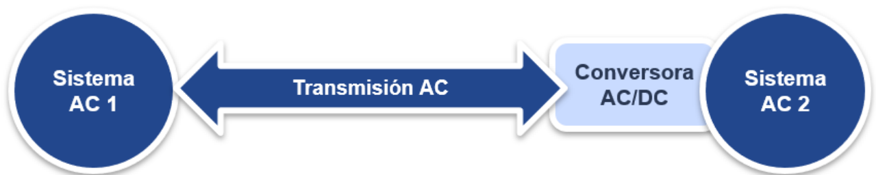
Figura 2.5: Conexión back to back.
