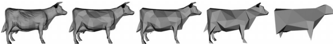
Figure 3.10: Sequence of simplifications made by the Garland-Heckbert algorithm. Image taken from Surface Simplification Using Quadric Error Metrics [8], Figure 4
