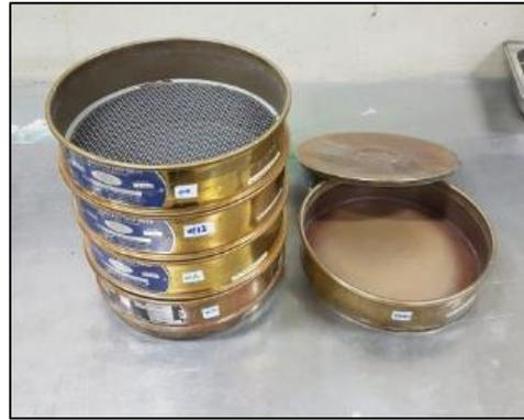
*Figura 62: "Tamices ASTM"*
