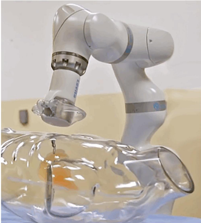
FIGURE 2 Model with free-standing robotic platform and intra-cavitary deployed magnetic grasper simulating tissue manipulation
