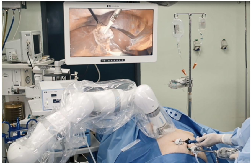
FIGURE 4 External view of the magnetic controller and internal view of the magnetic grasper
