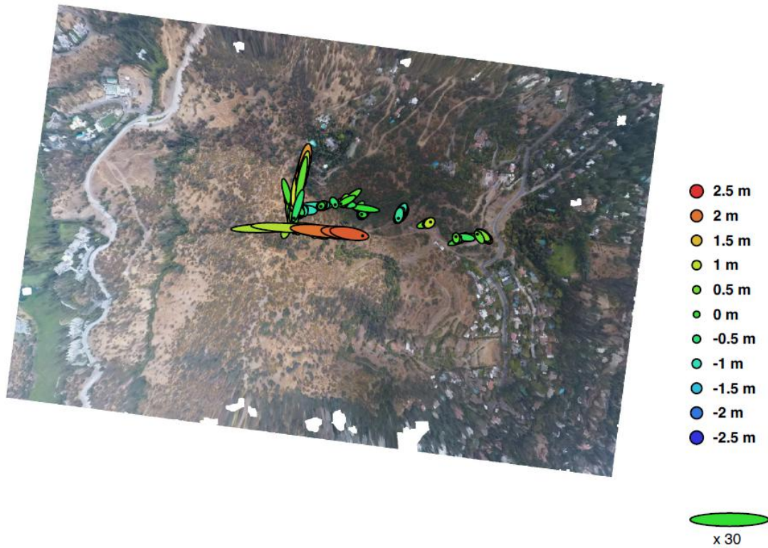
Figure 9.7 Camera locations and error estimates. Z error is represented by ellipse color. X, Y error are represented by ellipse shape. Estimated camera locations are marked with a black dot.
