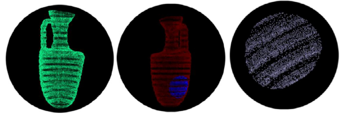
Fig. 16. On the left, the final point cloud obtained after the conversion used for the kd-tree FLANN method. On the center, the representative patch (in blue) no the model. On the right, final extracted patch. (For interpretation of the references to colour in this figure legend, the reader is referred to the web version of this article.)
