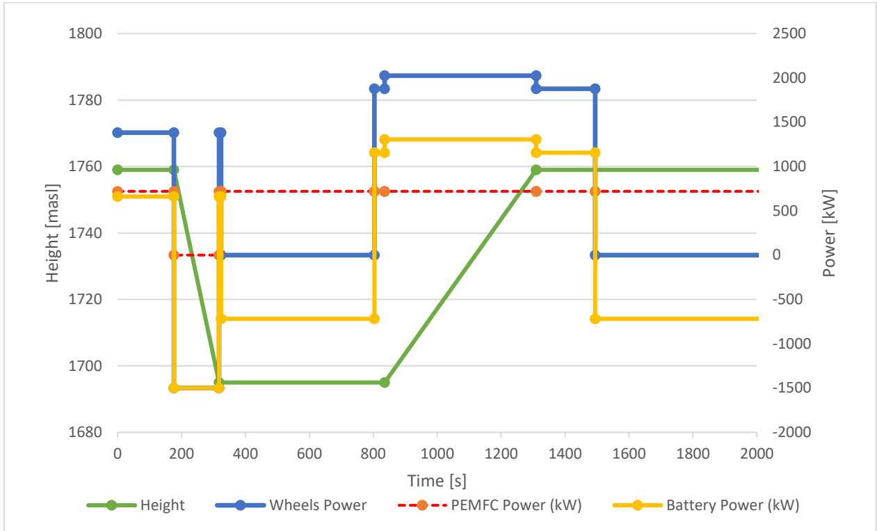
Figure 28: PEMFC, Lithium-Ion Battery and Wheels Powers projected through truck travelling time, compared with Height changes into the entire road over time.
