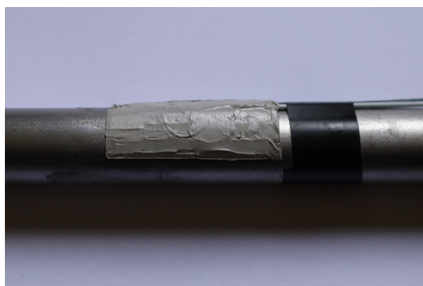
Figura 5.9: Coating del strain gage .
