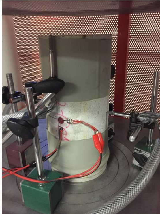
APPENDIX FIGURE A.6: SET-UP FOR 143 MM DIAMETER SPECIMENS
