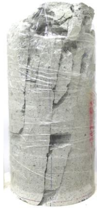
FIGURE 2.7: SAMPLE OF D = 143 MM TESTED WITH DIAMETRAL STRAIN CONTROL AT 0.001 MM/MIN DIAMETRAL STRAIN RATE
