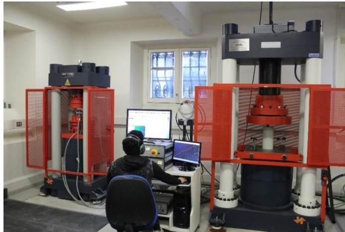
FIGURE 2.2: SERVO-ASSISTED PRESSES USED TO PERFORM THE UNIAXIAL COMPRESSION TESTS: ON THE LEFT, MES300 PRESS WITH 3,000 kN CAPACITY, AND ON THE RIGHT, MES800 PRESS, WITH 8,000 kN CAPACITY
