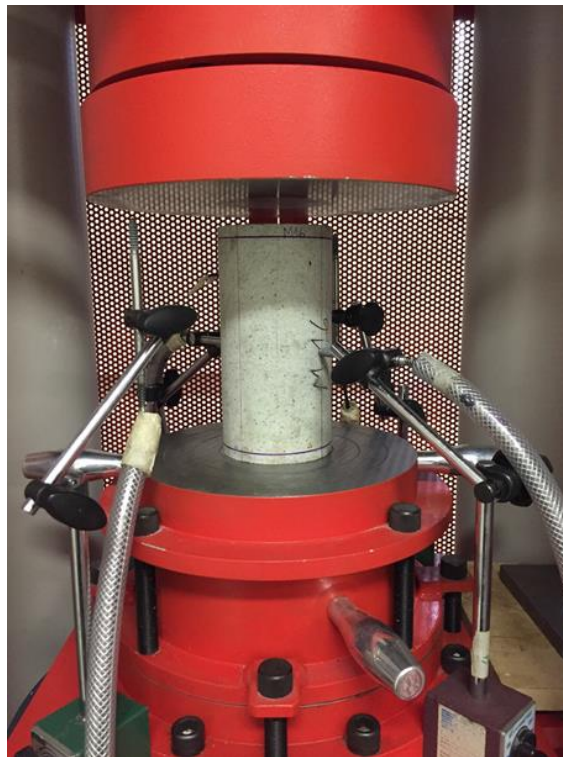
APPENDIX FIGURE A.5: SET-UP FOR 98 MM DIAMETER SPECIMENS
