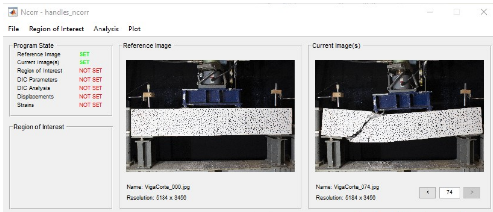
Figure B.1: Ncorr - Loading images procedure.
