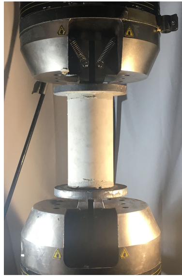
Figure A.3: Direct tensile test setup.
