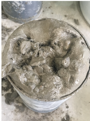
Figure 4.9: Concrete paste with PVA fiber.
