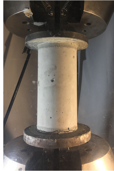
(b) Failure due to border conditions - PT2_03.
