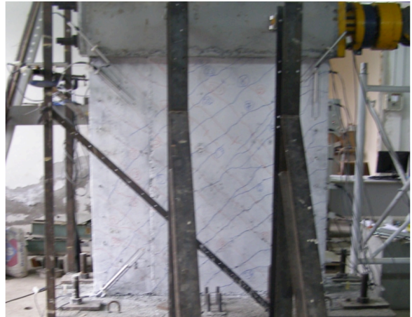
(b) Experimental cracking pattern (Terzioglu, 2011).
