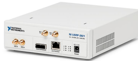
Figure 4.4: SDR used as sniffer of the communications
