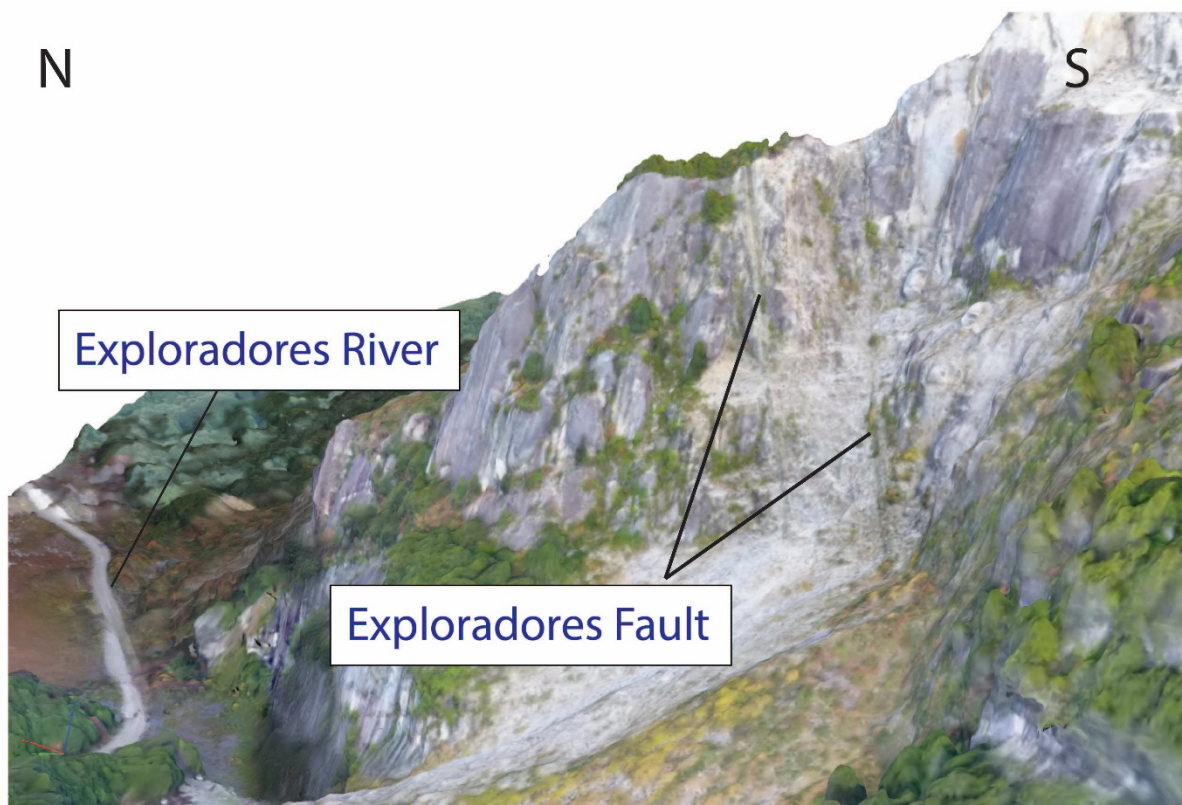
Figure 3.17. Screen capture looking east of structure from Motion (SfM) 3-D model of the Exploradores Fault along. Two parallel fault planes with fault breccia between them compose the fault core.
