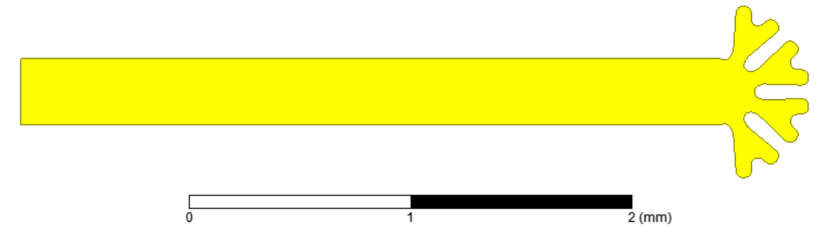
Figure 5.3: Detail of the probe designed for the Semi-Turnstile Version of the OMT. A metric scale is included.
