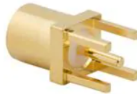
(d) Photograph of the considered coaxial connector.
