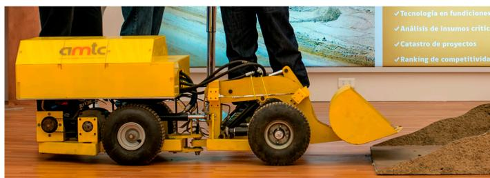
**Figure 12.** 1:5 scaled LHD built for testing and validation.
