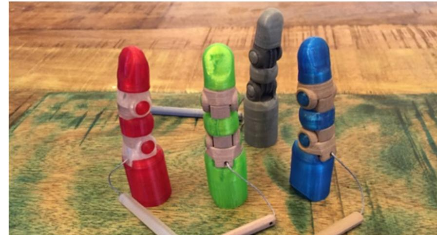
Imagen 18. Knick's Prosthetic Finger v3.5.
