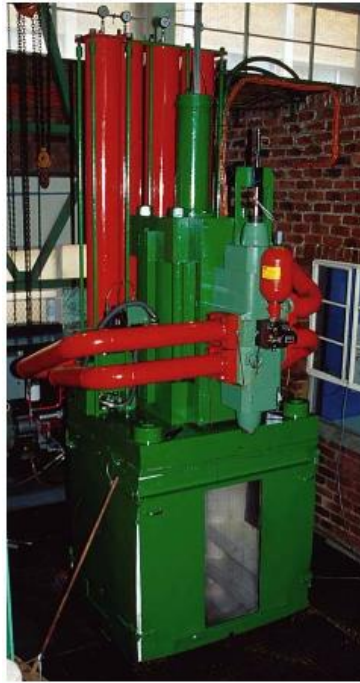
Figure 11 Terratek hydraulic equipment for dynamic tests. Taken from (Villaescusa et al., 2005a)
