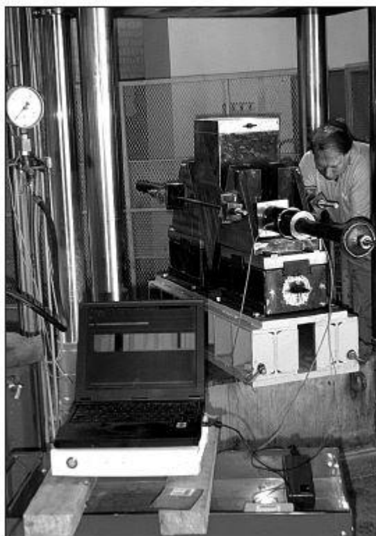
Figure 21 Block-wedge loading mechanism located under test facility (Ortlepp et al., 2005).
