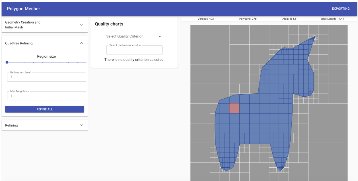
(b) After clicking on the polygon, it is subdivided into four new polygons.
