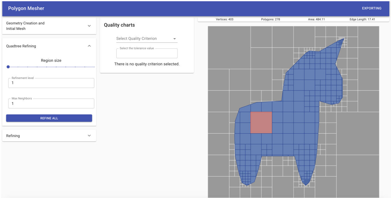
(a) The user places the cursor on the polygon that he wants to refine.
