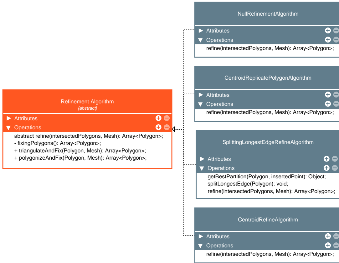
Figure 4.12: UML Diagram for refining algorithms.
