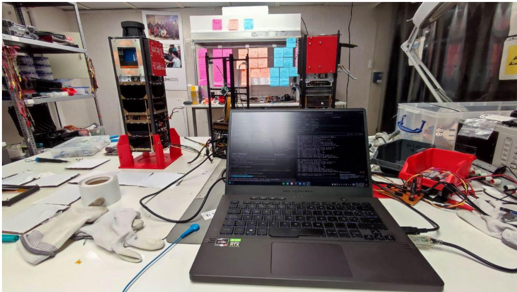
Figure 6.2: Laptop set up to run fuzz testing in a SUCHAI nanosatellite's main OBC through a serial communication interface.
