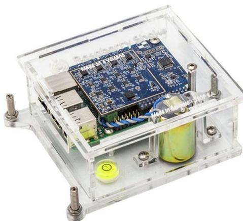
Figura 3.1: Sensor Raspberry Shake Indoor.
