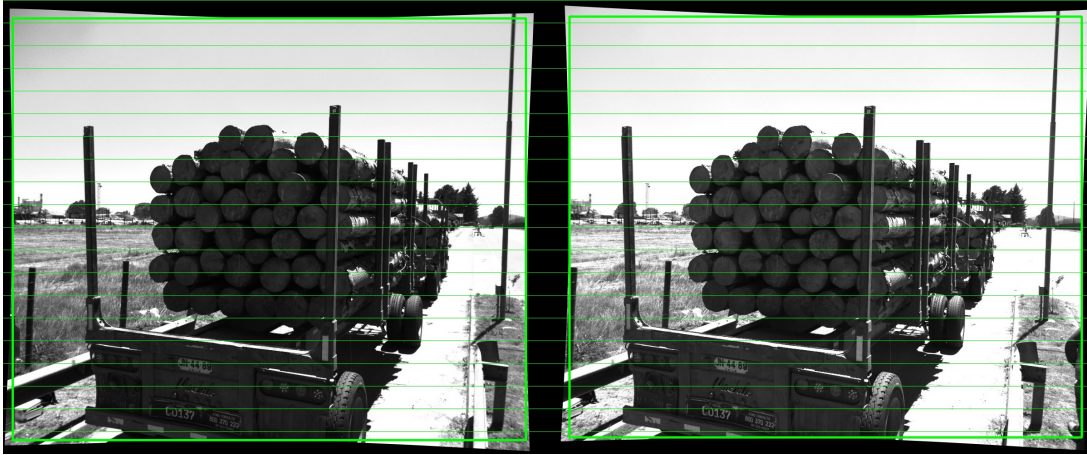
Figure 2.6: Figure 2.5 after rectification and calibration. Green lines correspond to the epipolar lines.
