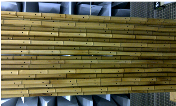
(a) Sonic crystals made of resonating bamboo rods [47].
