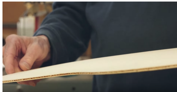
(b) An example of a finished double top soundboard. It is possible to observe the Nomex core between the two layers of wood.
