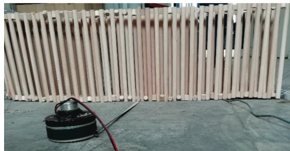
(b) Acoustic barrier made of cylindrical wooden bars [46].
