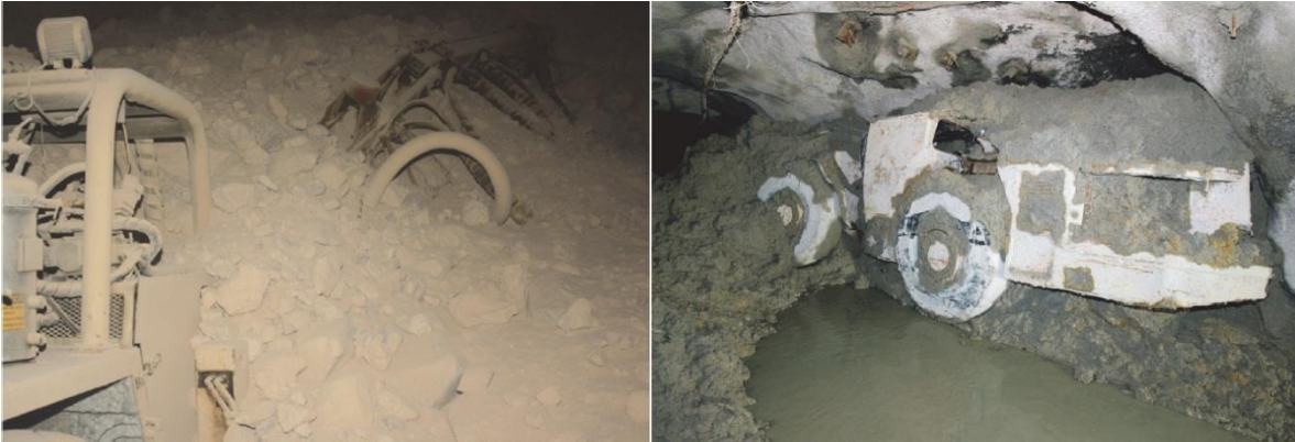
Figure 2.14 Inrush events in caving mines [124]. Left: Inrush of fine event. Right: Mud-rush event.
