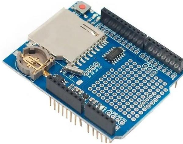
Figura 11. Data logging shield v1.0 [32]
