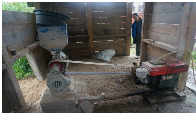
Figure 2.3 Small milling productive process powered by a diesel generator [49]
