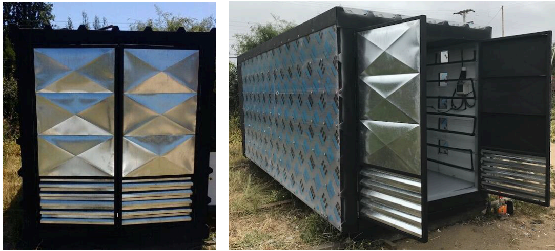
Figure E.7 Actual photos of the solar dryer [230]
