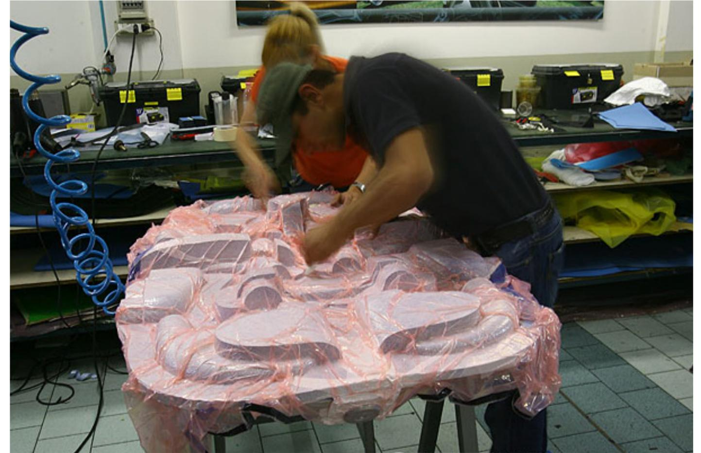
Figura 67: Laminado manual Pagani Huayra. Fuente: [http://www.speedhunters.com/2009/06/car\\_builder\\_gt\\_gt\\_pagani\\_factory\\_tour\\_pt\\_2/](http://www.speedhunters.com/2009/06/car_builder_gt_gt_pagani_factory_tour_pt_2/)
