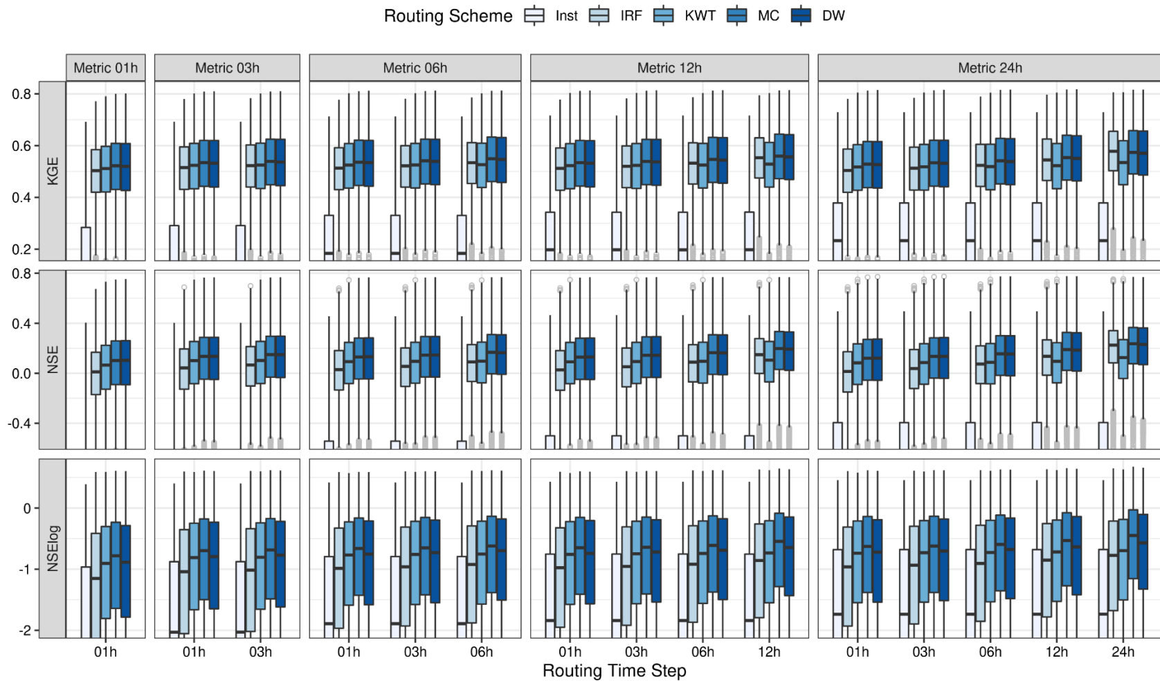
Figure 5. Impact of routing scheme and routing time step on performance metrics (rows) computed for the period April/2008-March/2012, using different discharge temporal resolutions (columns) across a large sample of VIC parameter sets obtained through Latin Hypercube Sampling (see text for details). The results are presented for instantaneous runoff (Inst), Impulse Response Function (IRF), Kinematic Wave Tracking (KWT), Muskingum-Cunge (MC) and Diffusive Wave (DW).
