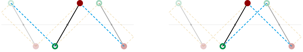
Fig. 4.6: The unit cell used before includes one spring at each side of the bar(left), now we will take a chain that includes both springs at right-side(right).
