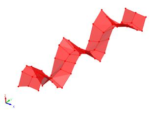
**Figure 9.** Initial state mode shape  $\omega = 278.38$  Hz.
