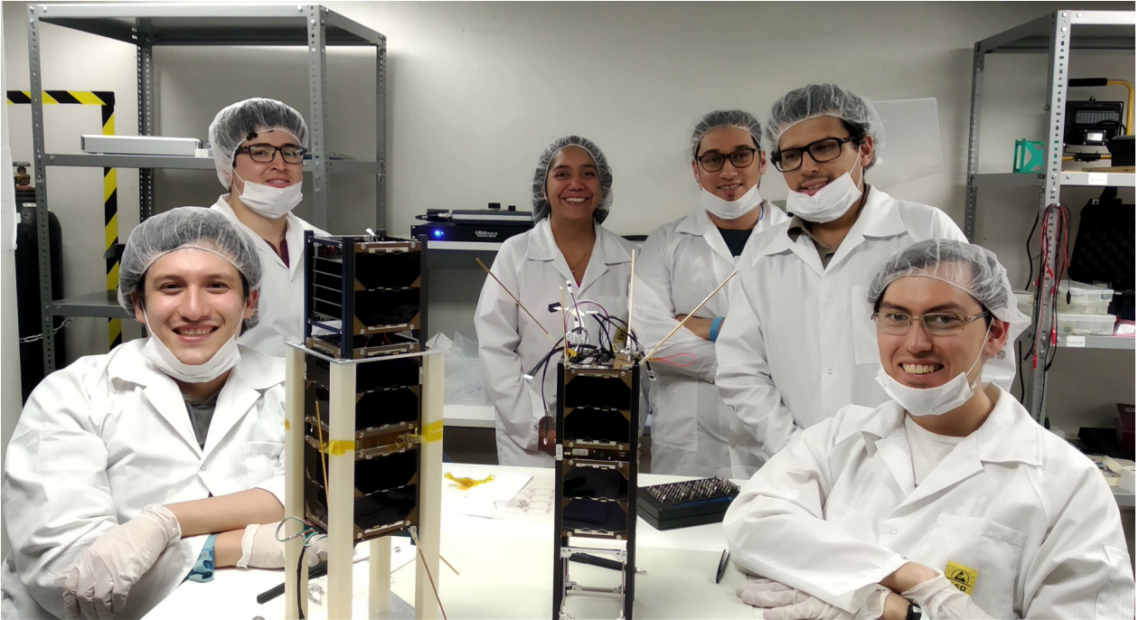
Figure 1.1: Images of the SUCHAI-2 and -3 CubeSats during the integration process together with part of the development team at the Space and Planetary Exploration Laboratory (SPEL). These CubeSats were launched on April first, 2022. They carry magnetometers and an S-band communication system to receive the data from a femto-satellite. The femto-satellite also has a magnetometer, and it will be carried and deployed by the SUCHAI-3 CubeSat. I am studying the feasibility of estimating the location of a radio source (femto-satellite) in a concrete scenario, in low earth orbit where there are only two CubeSats available to estimate the location of a femto-satellite.
