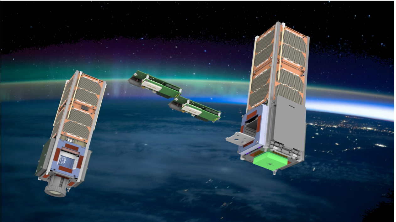
Figure 3.1: The goal of this Thesis is to evaluate the possibility of estimating the position of a femto-satellite using only two CubeSats. Although I did my research using simulations, I took elements of an actual situation. We have two CubeSats in space with Star Trackers, GNSS receivers, S-band transceivers, and antenna arrays. Most importantly, we have a Femto-satellite Orbital Deployer (FOD) with a femto-satellite on board the SUCHAI-3.
