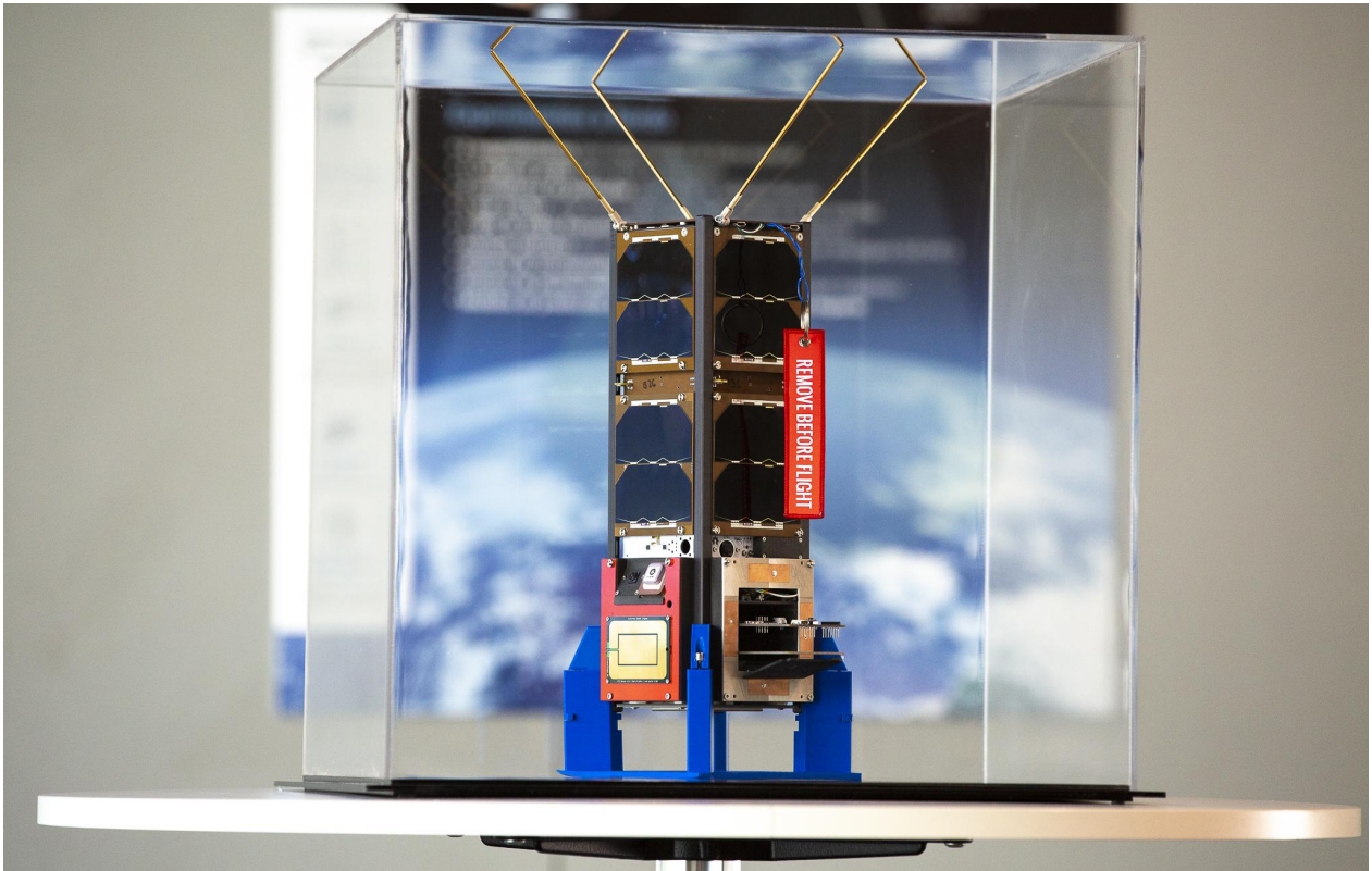
Figure 3.3: A 3U CubeSat has enough space to have femto-satellites and a deployment system for the femto-satellites. This picture shows the SUChAI 3 carrying two femto-satellites.
