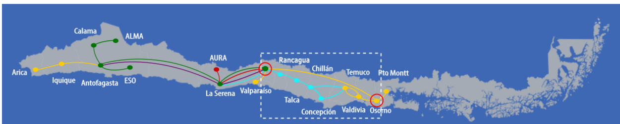
Figure 3.5: Example of nodes becoming transit networks over the Chilean’s National University Network (REUNA 2018 [32]). Consider the Santiago and Osorno nodes circled in red. If the yellow link between them fails, all communications between these cities needs to be re-directed between the remaining nodes inside the white rectangle.
