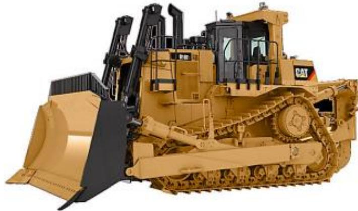
**Figura 5: Bulldozer D10T, Caterpillar.**
