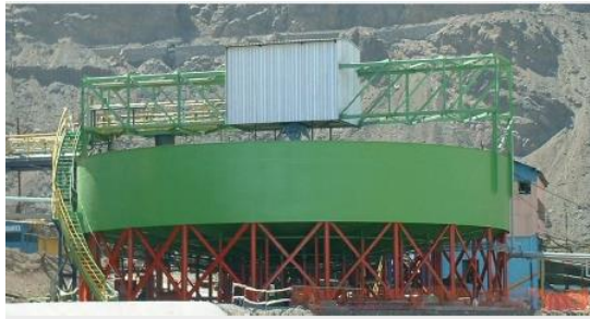
Concentrate Thickener, 21m diameter High Rate E-DUC® Auto Dilution System Bridge Type Elevated Tank
