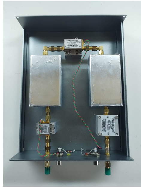
(b) Top view microwave receiver
