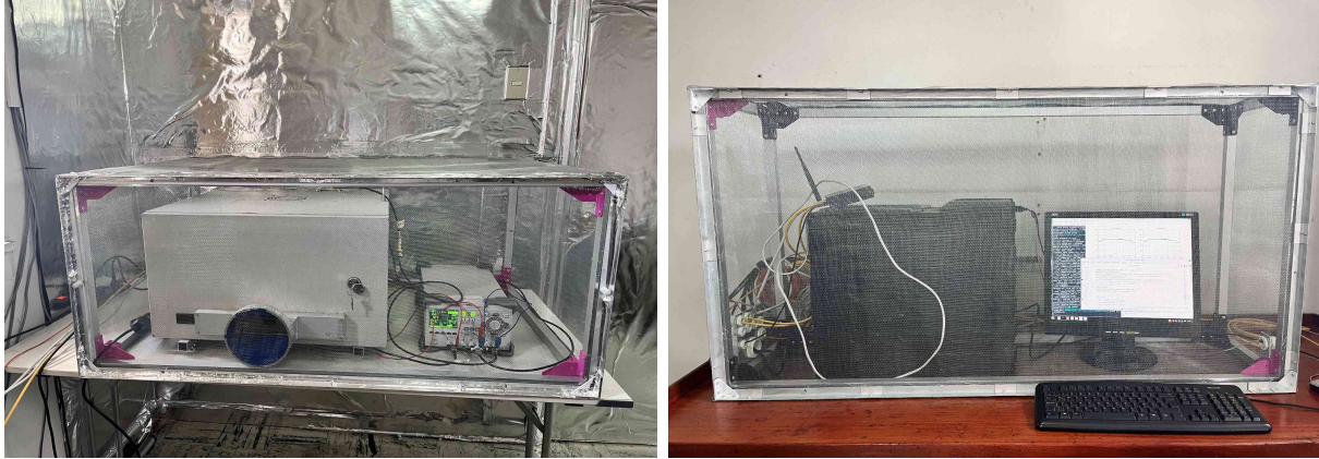
(a) Receiver, ROACH2 and power supply.
