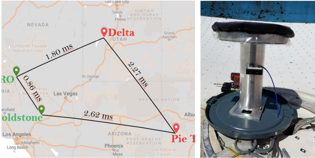
Figure 2.7: Left: The green zones, OVRO and Goldstone, represent operational sites with a travel time between them of 0.86 seconds. The red zones, on the other hand, are potential sites for future operational stations. Right: Choke-ring feed located at OVRO [1].
