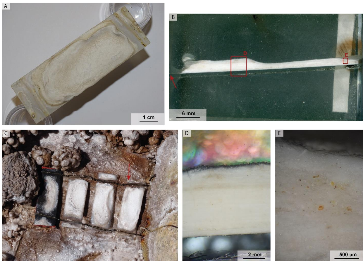
Figure 54: (A) Sample VR03-52 from point VR03 at Vega Rinconada, showing the whitish precipitate with light brown tones. (B) Polished cross section of A, indicating the position of samples D and E obtained by optical microscopy. The red arrow indicates the same position as in image C. (C) Image of the day of sample extraction (22-04-2023), all slides show precipitated material. The vent is located upwards with respect to the image. (D) Close-up of the image in B, an almost homogeneous layer of precipitated opal is observed, with a slight presence of very small detritus. (E) Close-up of the image in B, it is observed that the precipitate is almost massive without laminations, besides the yellowish detritus that were cemented.
