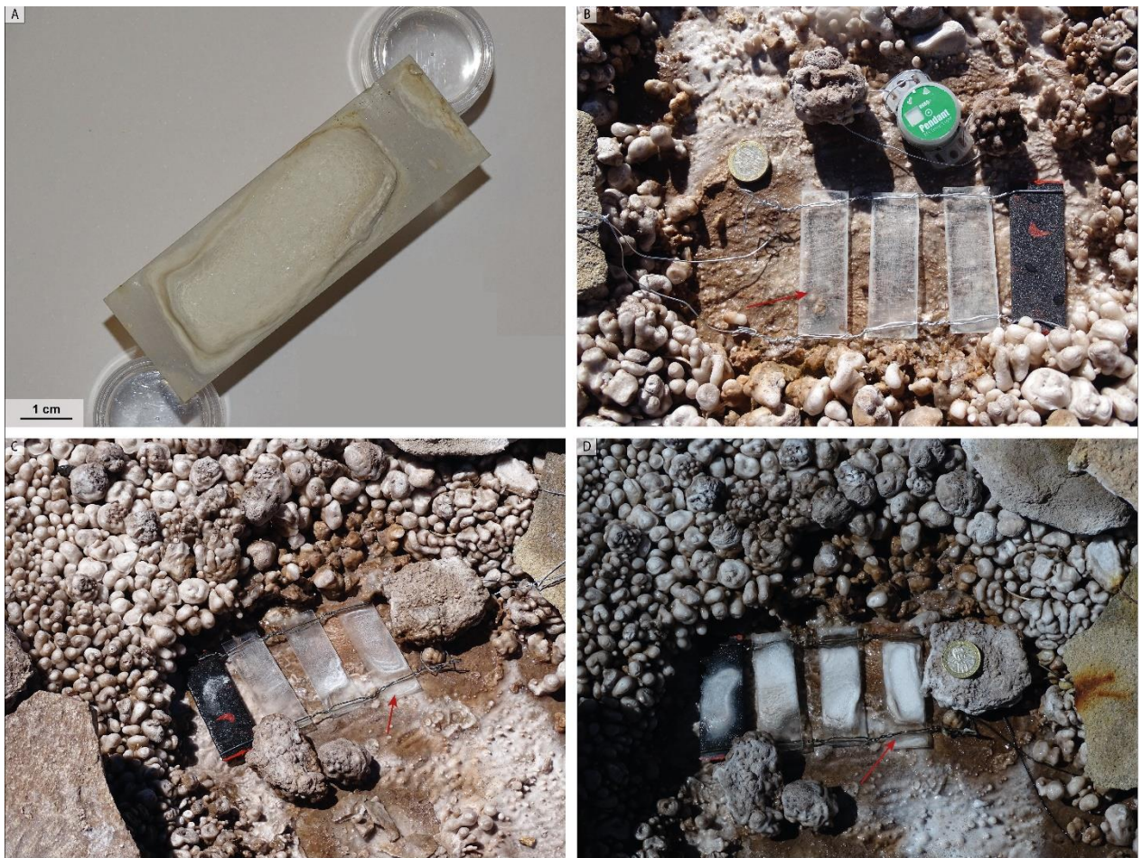
Figure 53: (A) Sample VR03-27 from point VR03 of Vega Rinconada, used for the representative chemical analysis. (B) Image of the day of sample installation (25-09-2021), the red arrow on the left indicates the position of the slide, also a Chilean 100 pesos coin is presented as scale. The vent is located downwards with respect to the image. (C) Image a few days later (01-10-2021) where it is observed that some silica precipitated in the samples, the red arrow indicates the position of the sample in A and the vent is located towards the upper left zone with respect to the image. (D) Image on the day of sample extraction (22-04-2022) showing that all the slides have precipitate. The red arrow indicates the position of the sample in A, there is also a Chilean 100 pesos coin as a scale, and the vent is located upwards with respect to the image.
