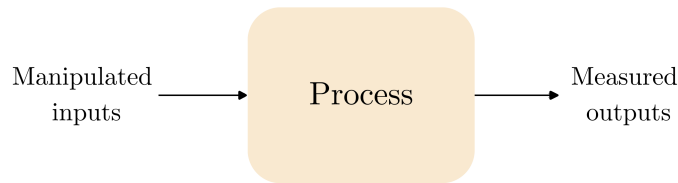
(a) Open-loop representation of a control system
